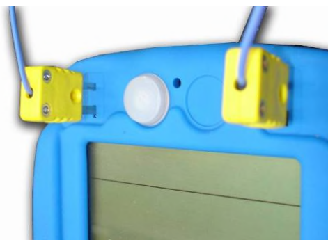
Connecting temperature probes
